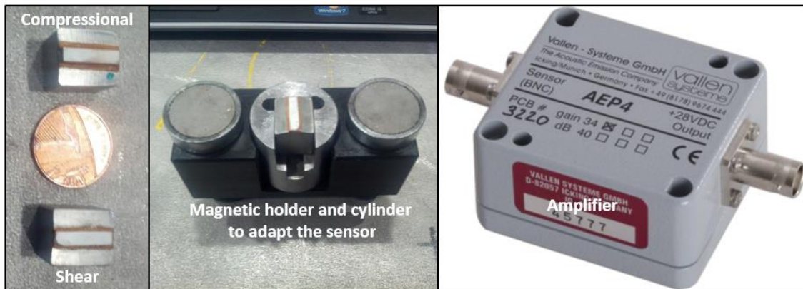
Figure 6-19 Sensors (left), Magnetic holder (centre), Amplifier (right)
