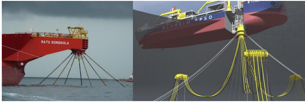
Figure 1-2 Single point external turret (left) Submerged turret production (right) [7]
