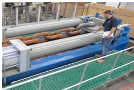
Figure 8-6 Fatigue chain tensile test
