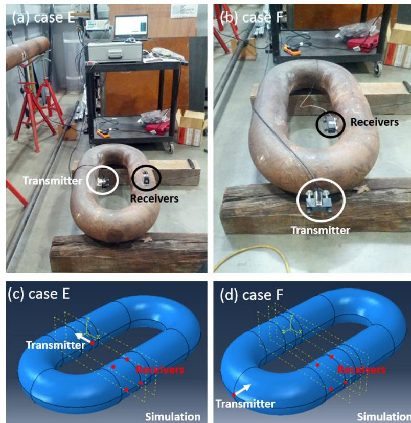
Figure 7-23 Experimental set-up and simulation case for chain link of large diameter
