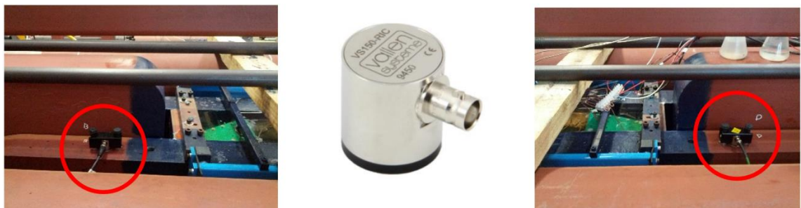
Figure 3-4 AE sensor type VS150-RIC (left: sensor 3, right: sensor 1)
