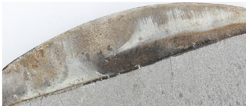
Figure 3-13 Notch and crack growth (left), zoom of crack growth (right).
