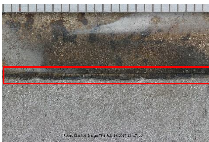
Figure 3-14 Crack growth (inside red colour)
