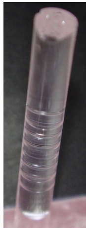
FIGURE 7.20: CO 2 laser-machined resonators on sample R75. Resonators are numbered 1-5 from the top.
