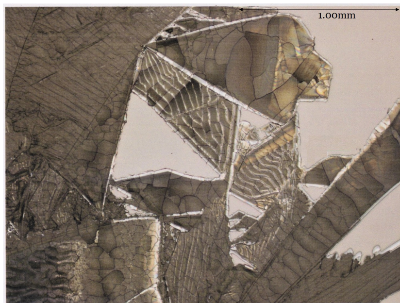
FIGURE 5.3: Cracking of the surface layer of sample NB223-1, protected using SU-8 negative photoresist and hydrogen-loaded before being UV written.
