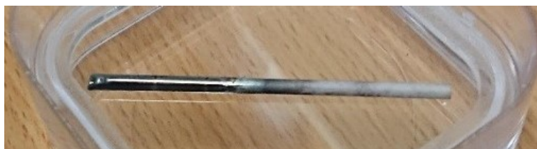
FIGURE 6.12: Rod R79 after annealing at 500 °C in a hydrogen-only atmosphere.
