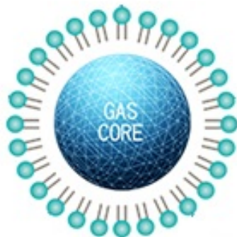
Figure 1.8: The figure shows the monolayer structure of a microbubble shell. Phospholipids organise spontaneously so that their hydrophobic acyl chains face the gas core, and their hydrophilic headgroups face the surrounding aqueous environment of the bubble. [50]
