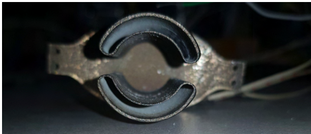
Fig. 14 Hollow anode condensation - thruster OFF.
