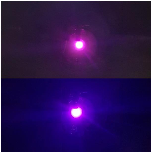
Fig. 28 Plume of the CHT-Zn on zinc: (up) electro-magnets off; (down) electromagnets on;
