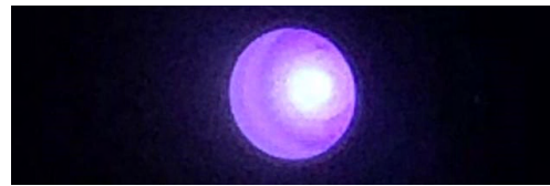
Fig. 24 CHT-Zn channel during operation.
