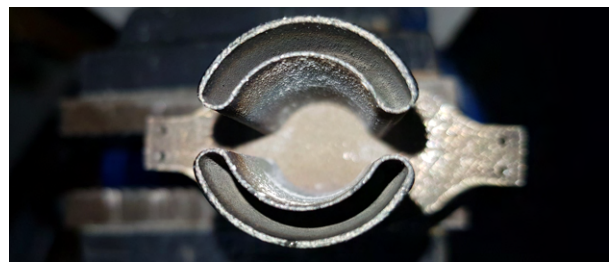
Fig. 15 Hollow anode condensation - thruster ON.
