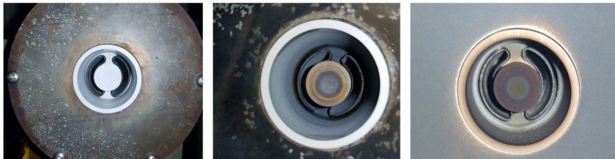
Fig. 40 Channel deposition: (left) new channel; (middle) deposition with krypton and zinc mixture; (right) deposition after sustained zinc operation;
