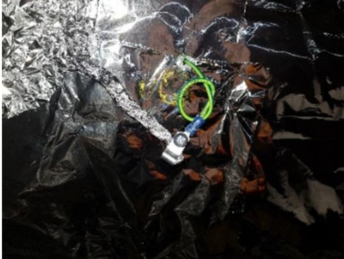
Figure 7.6: The way to connect aluminium foil with a cable. Cable has only a ground wire inside. The cable is led outside of the booth through the hole drilled in the wall and switched to the socket.
