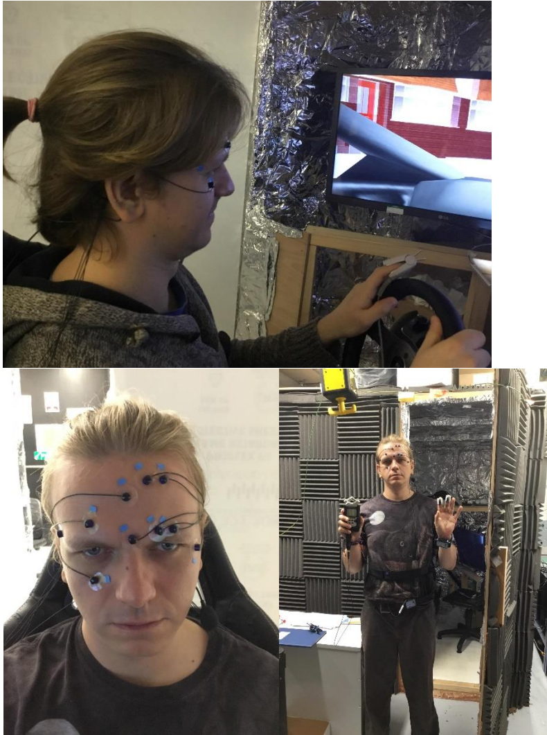
Figure 8.7: Experimental set-up of the participant allocated to group 2 with EOG and forehead EMG measurements.
