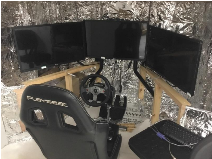
Figure 8.4: The set-up of the driving simulator inside the Faraday Cage.
