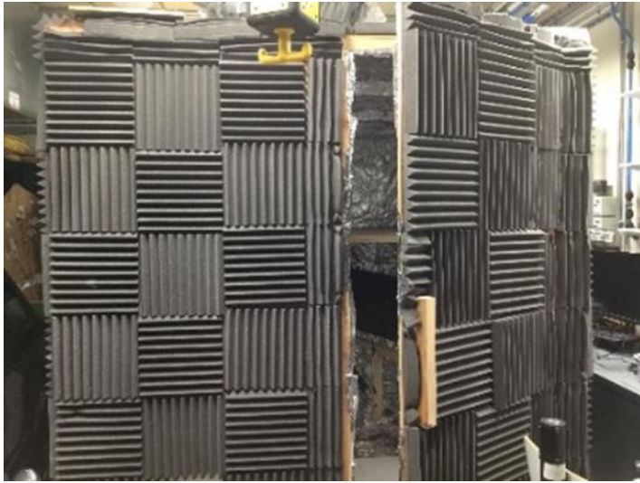
Figure 7.4: Outside of the laboratory booth insulated with fire-retardant acoustic foam to reduce acoustic noise in the voice recording.
