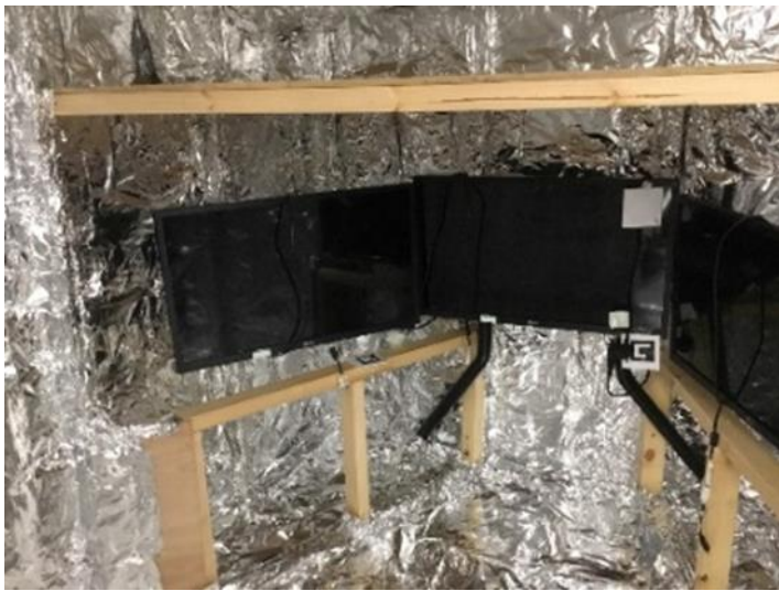
Figure 7.5: Inside of the laboratory booth insulated from electromagnetic noise with several layers of a heavy-duty aluminium foil.
