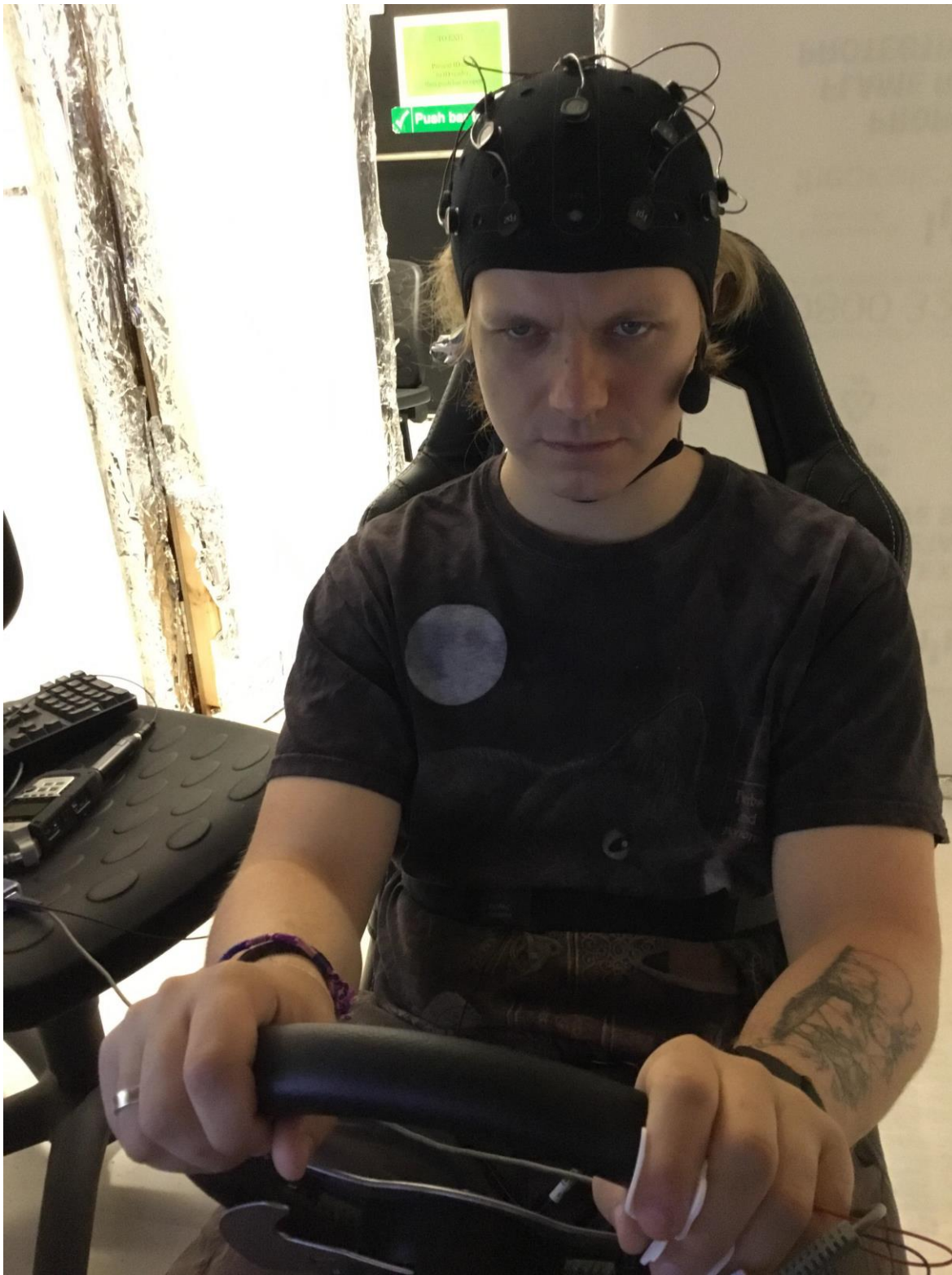
Figure 7.2: : Participant driving a driving simulator with EEG cap on the head, EDA electrodes and oximetry sensor on the fingers. It is also visible that he has a respiration belt around the abdomen and a head-mounted microphone. The ECG electrodes are hidden under the t-shirt.
