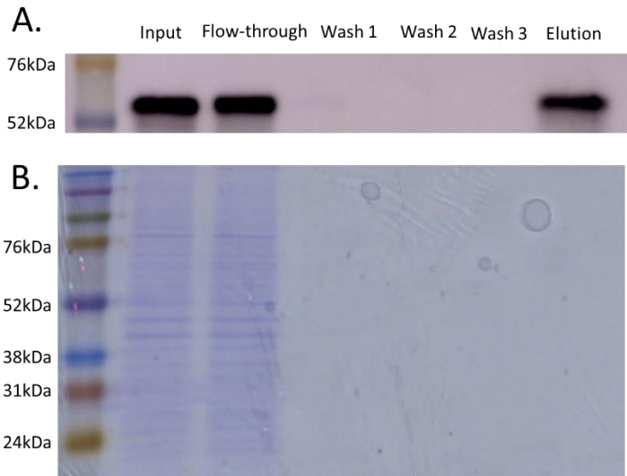
Figure 5.7: Western blot and Coomassie stain of GFP-trap co-immunoprecipitation of full-length GFP-tagged WISP-1. A. Western blot using anti-GFP antibody of lysates from HEK- 293T cells expressing GFP-tagged full-length WISP-1. Input is cell lysate, flow-through is what remains in the lysate after incubation with the beads, washes 1-3 are taken from washes with bead dilution buffer, and elution is the final elution using the kit elution buffer. Expected molecular weight of WISP-1-GFP is 73kDa. B. Coomassie brilliant blue staining of the gel from A, showing protein staining.
