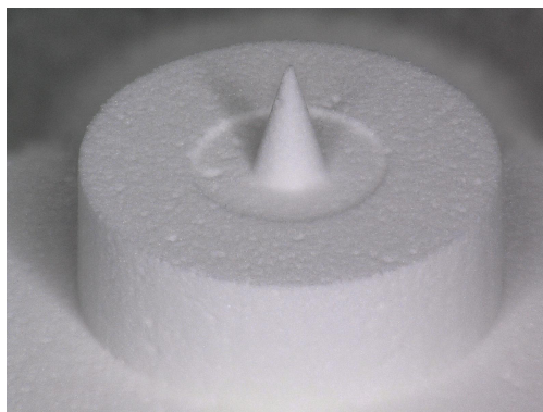
Fig. 2 Image of the type of porous borosilicate single emitter used during testing.
