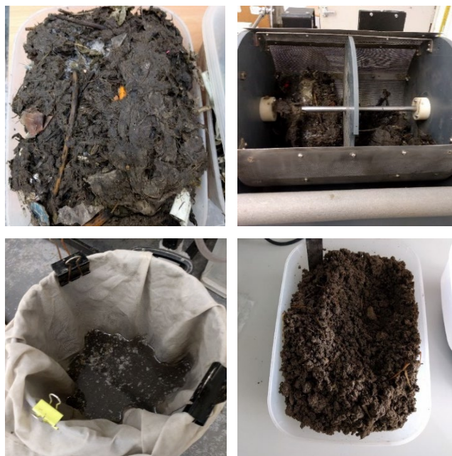
Image 1. ORS formation steps. Top left: pulped OFMSW. Top right: washing process. Bottom left: filtering wash water. Bottom right: drained ORS
