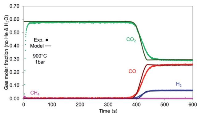
Fig. 13 Gases breakthrough for reduction with synthetic biogas (CO<sub>2</sub> : CH<sub>4</sub> = 6 : 1) for 900 °C and 1 bar.
