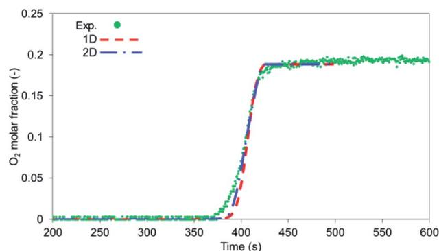
Fig. 6 O<sub>2</sub> breakthrough comparison between the experiment (circular markers) and 1-D model (red dashed line) and radially averaged 2-D model (blue dashed dotted line), flow rate 10 NLPM, bed temperature 600 °C and pressure 1 bar.
