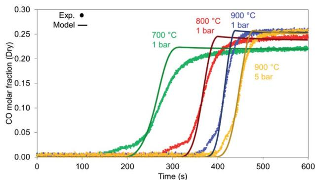
Fig. 15 CO breakthrough during reduction for various bed temperatures and pressures for reduction with synthetic biogas  $\text{CO}_2 : \text{CH}_4 = 6 : 1$  for  $900\text{ }^\circ\text{C}$  and 1 bar.
