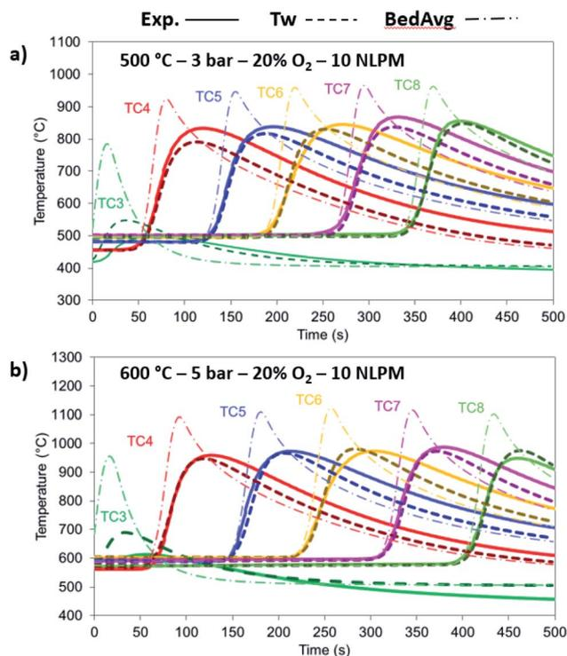
Fig. 8 Comparison between the experimental (solid lines), 1-D thermowell model (dashed lines) and 1-D bed model (dashed dotted lines) temperature for 20% O<sub>2</sub> and 10 NLPM with (a) 500 °C/3 bar and (b) 600 °C/5 bar.
