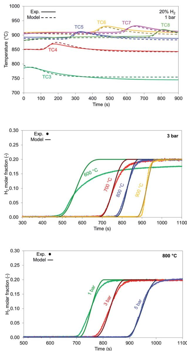
Fig. 11 (Top) Temperature profiles for the experiment (solid lines) and model (dashed lines) for reduction with 20% H<sub>2</sub> at 900 °C, 1 bar and 10 NLPM; (middle) temperature comparison for H<sub>2</sub> breakthrough during reduction with 20% H<sub>2</sub> at 3 bar pressure and 10 NLPM flow rate; (bottom) pressure comparison for H<sub>2</sub> breakthrough during reduction with 20% H<sub>2</sub> at 800 °C and 10 NLPM flow rate.
