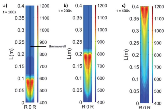
Fig. 5 2-D model radial profiles for 20% O<sub>2</sub>, 600 °C set bed temperature and 1 bar pressure at 100 seconds (a), 200 seconds (b) and 400 seconds (c).
