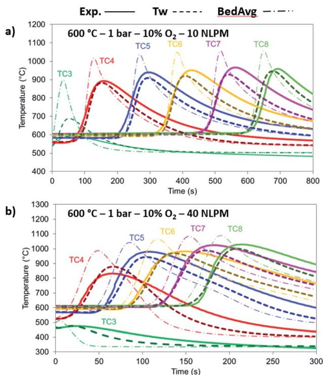
Fig. 10 Temperature comparison between the experimental (solid lines), 1-D thermowell model (dashed lines) and 1-D bed model (dashed dotted lines) temperature for 10% O<sub>2</sub>, 1 bar and 600 °C with (a) 10 NLPM and (b) 40 NLPM.
