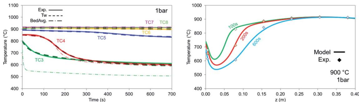
Fig. 17 (Left) Dry reforming temperature profiles for the experiment (solid lines), thermowell model (dashed lines) and bed average (dashed dotted lines). Conditions are 900 °C, 1 bar, 12 NLPM and  $\text{CO}_2 : \text{CH}_4 - 6 : 1$  balanced with He. (Right) Axial temperature profiles for dry reforming for the experiment (diamond markers) and model (solid lines), at 900 °C, 1 bar, 12 NLPM and  $\text{CO}_2 : \text{CH}_4 - 6 : 1$  balanced with He.
