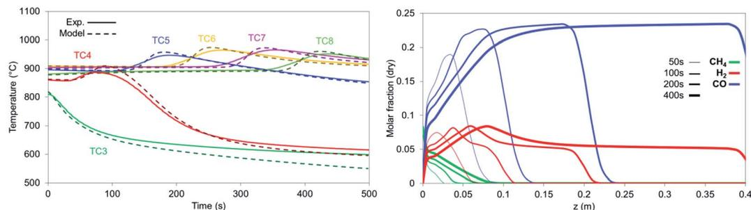
Fig. 14 (Left) Temperature profiles for the experiment (solid lines) and model (dashed lines) for reduction with synthetic biogas ( $\text{CO}_2 : \text{CH}_4 = 6 : 1$ ) for  $900\text{ }^\circ\text{C}$  and 1 bar. (Right) Axial molar fraction profiles during reduction with synthetic biogas  $\text{CO}_2 : \text{CH}_4 = 6 : 1$  for  $900\text{ }^\circ\text{C}$  and 1 bar.
