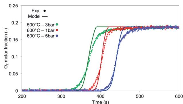
Fig. 7 O<sub>2</sub> breakthrough comparison between the experiments (circular markers) and 1-D model (solid lines), at a flow rate of 10 NLPM.
