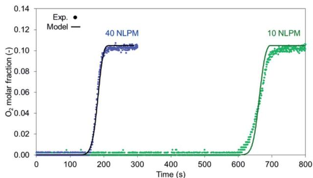
Fig. 9 O<sub>2</sub> breakthrough for a high flow rate (40 NLPM – 1 m s<sup>-1</sup>) and lower flow rate (10 NLPM – 0.1 m s<sup>-1</sup>).
