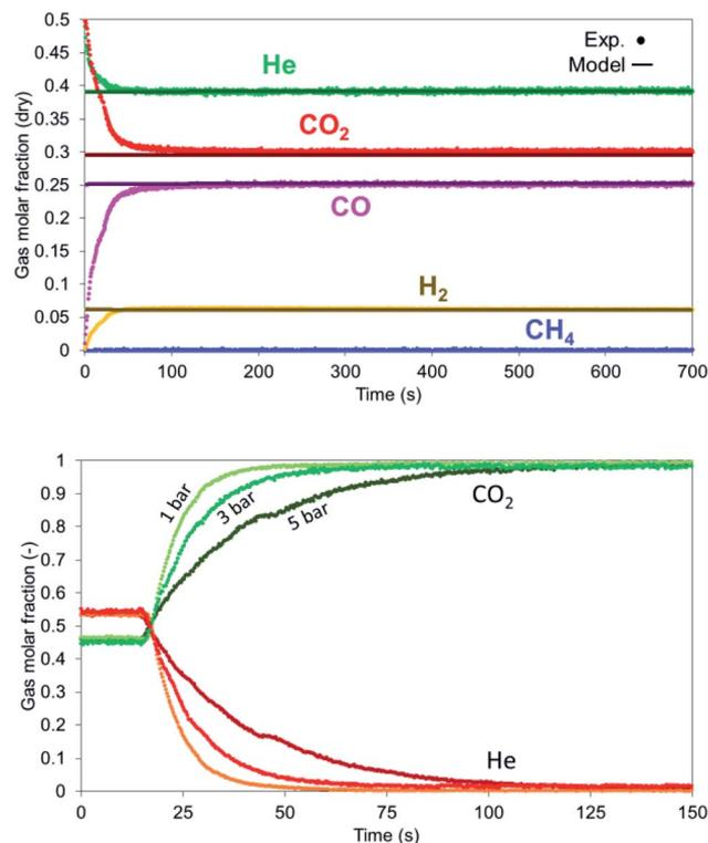
Fig. 16 (Left) Gas profiles during dry reforming at  $900\text{ }^\circ\text{C}$ , 1 bar, 12 NLPM flow rate and  $6 : 1 - \text{CO}_2 : \text{CH}_4$ . (Right) Dispersion effect at various pressures on the gas detection for a mixture of He and  $\text{CO}_2$ . He valve is switched off at 20 seconds.
