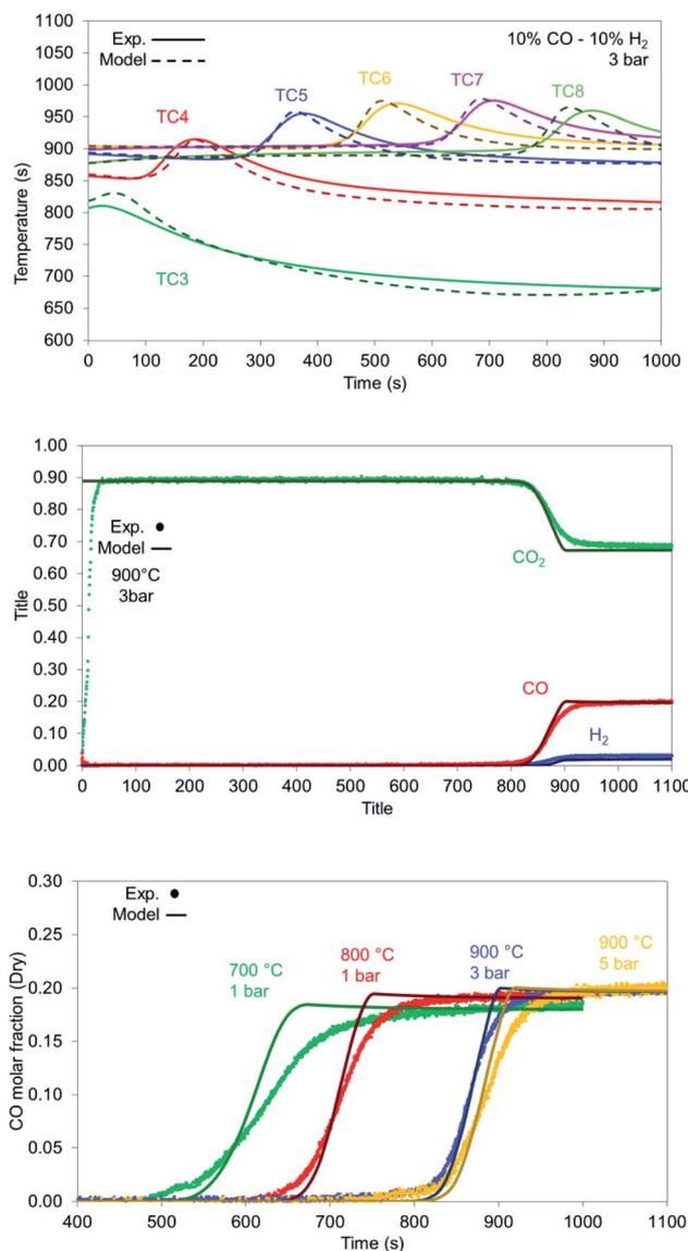
Fig. 12 (Top) Temperature profiles for the experiment (solid lines) and model (dashed lines) for reduction with 10% H<sub>2</sub>, 10% CO and 70% CO<sub>2</sub> at 900 °C, 3 bar and 10 NLPM; (middle) gas breakthrough for reduction with 10% CO, 10% H<sub>2</sub> and 70% CO<sub>2</sub> (no He and H<sub>2</sub>O); (bottom) CO breakthrough during reduction for various bed temperatures and pressures for reduction with 10% CO, 10% H<sub>2</sub> and 10 NLPM flow rate.
