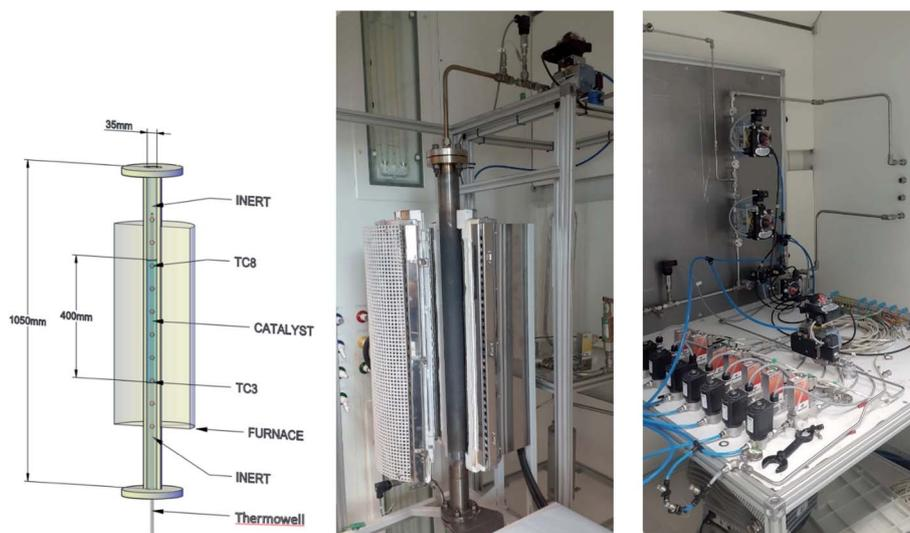
Fig. 2 (Left) CLR packed bed reactor schematic; (center) packed bed reactor system placed in FC-2 at the University of Manchester; (right) gas feeding system placed in FC-1.<sup>38</sup>
