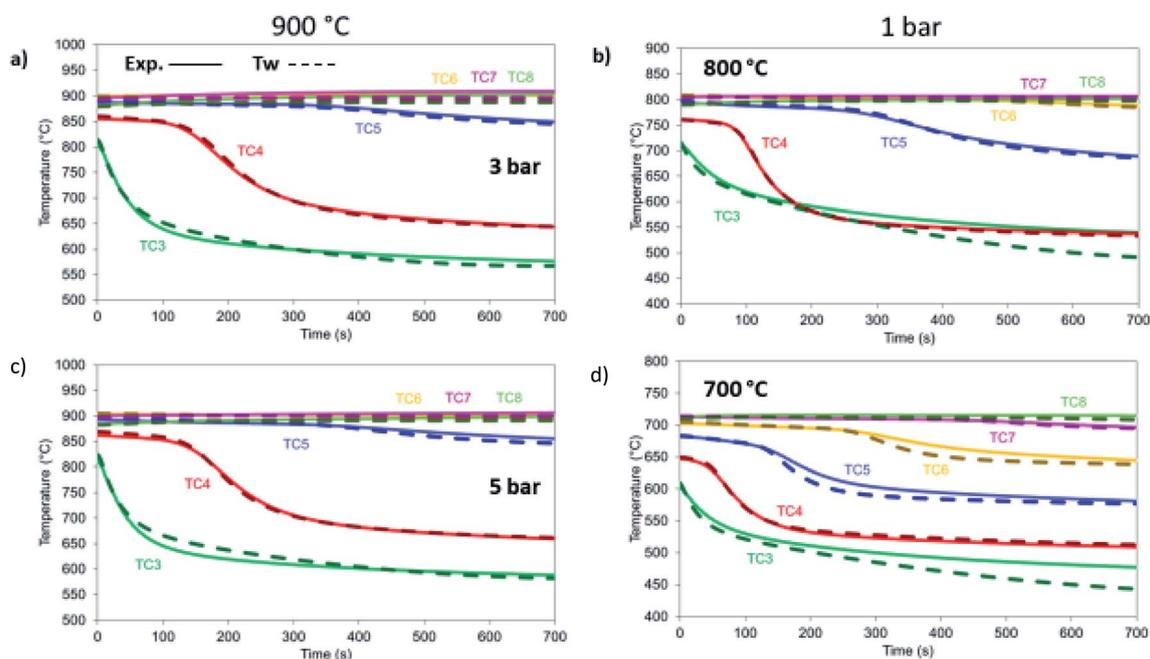
Fig. 18 Dry reforming under different temperature and pressure conditions. All cases are 12 NLPM, 6 : 1  $\text{CO}_2 : \text{CH}_4$  and balanced 8 with He: (a) 900 °C, 3 bar, (b) 800 °C, 1 bar, (c) 900 °C, 5 bar, (d) 700 °C, 1 bar.
