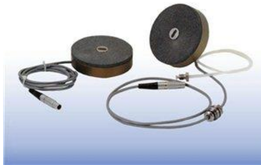
Figure 100: 100mm dia. bender elements in top and bottom caps (VJtech, 2015)
