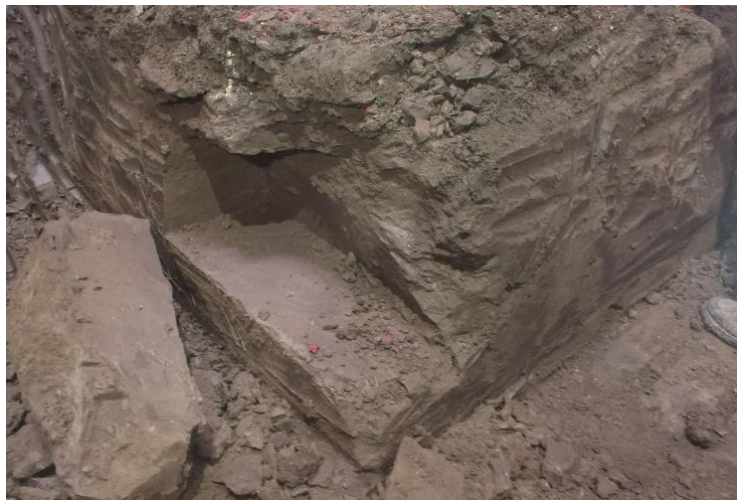
Figure 112: Failure along an existing fracture
