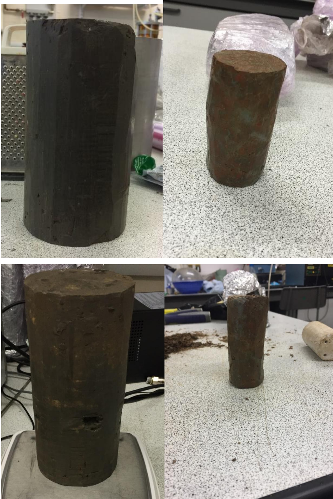
Figure 115(a-d): During trimming of samples, near completion. a) London Clay Unit B2 100mm dia. b) Lambeth Group UMB 38mm dia. c) London Clay Unit A2 100mm dia. d) UMB 38mm dia.
