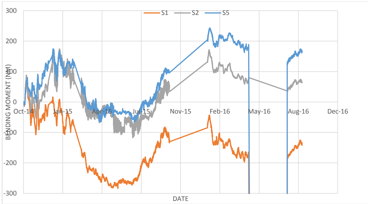
Figure 79: Bending moments corrected for temperature fluctuations East-West (+/ve shows sag, -/ve shows tension)
