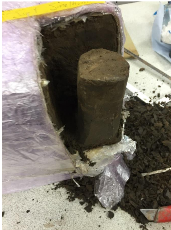
Figure 114: Initial trimming of a sample from block
