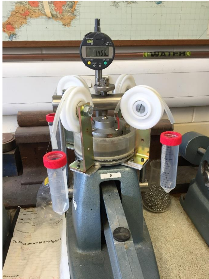
Figure 90: Oedometer with counter-pulley system
