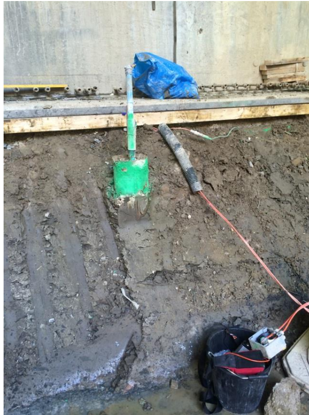
Figure 58: Exposed instrumentation on slope. The spade (green) is placed within the photograph as a reference point. Photo shows a pressure cell partially destroyed at the top of the slope with a shallow piezometer connected to a datalogger (held in a bucket).
