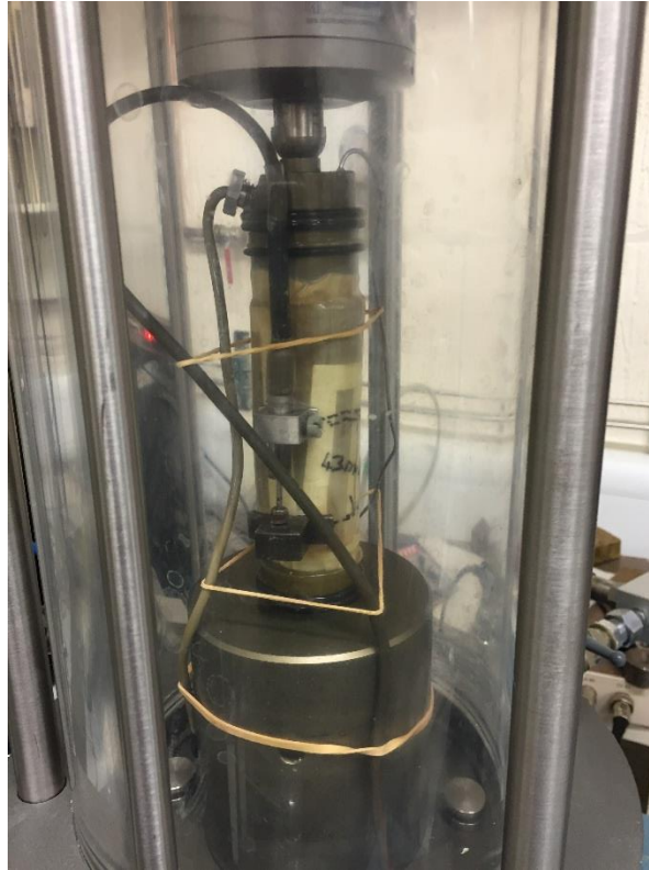
Figure 117: Sample pressurised in the 38mm diameter triaxial cell and ready for testing
