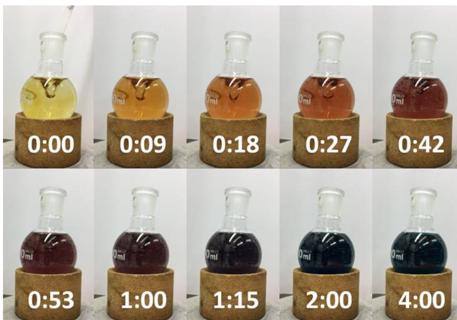
Figure 2.11 Change in colour over time for a 100 mL batch synthesis of AgNPs.
