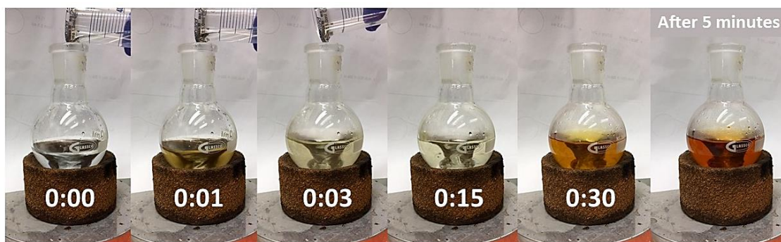
Figure 2.20 Batch reaction filmed to observe the relative colour variations. Time frame were captured as indicated in the figure. Volume ratio water:IPA was of 1:1.
