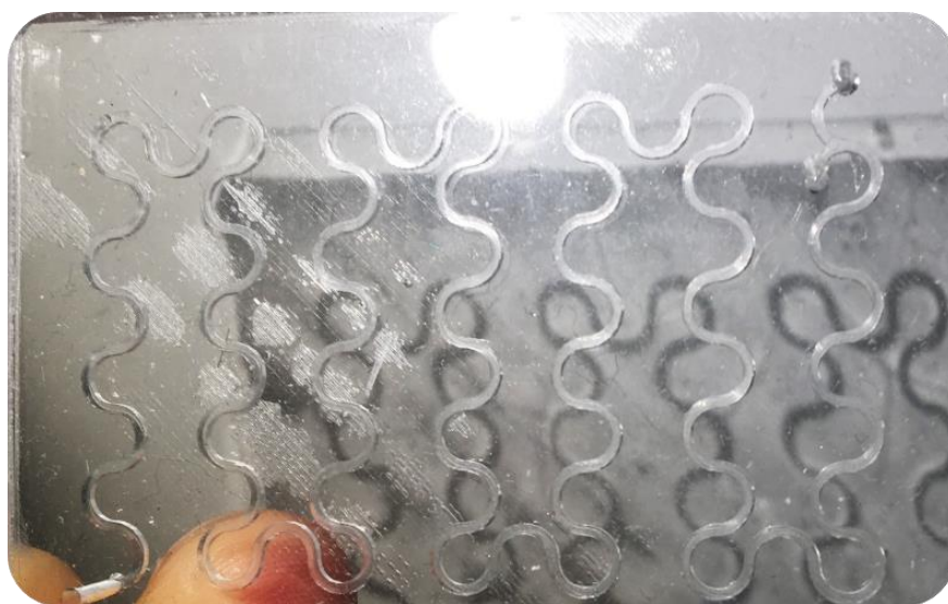
Figure 4.25 two inlet curved serpentine replica mould casted device, bonded on PDMS by oxygen plasma treatment (3DP-RMC*PDMS)
