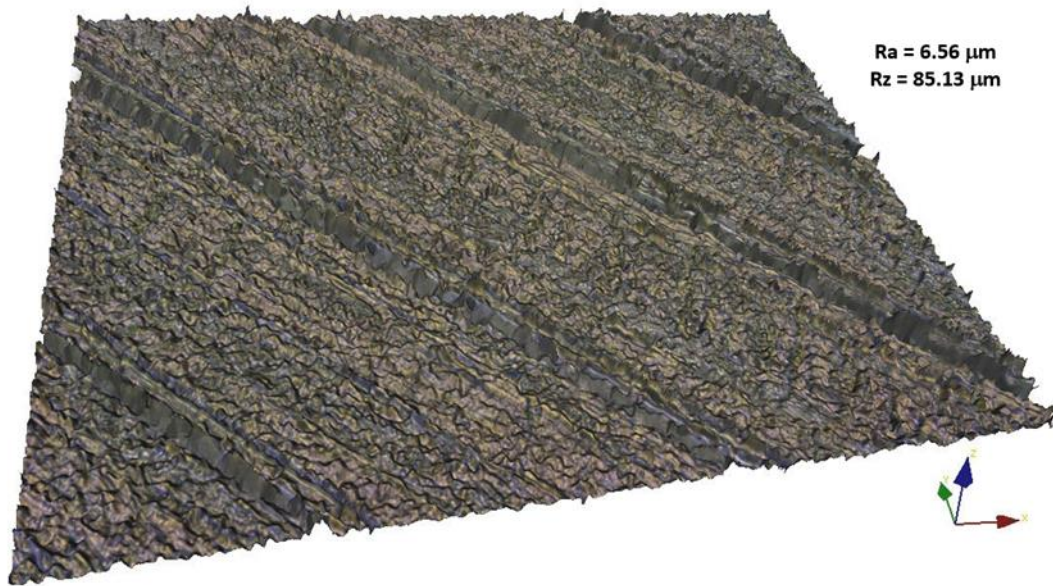
Figure 3.20 Morphological characterisation of the 3D printed base including average roughness (Ra) and maximum peak-to-peak value (Rz).
