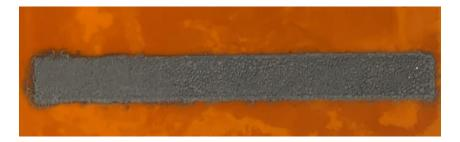
**Fig. 5.6**- Image of 5 x 50 mm PVDF- $Bi_{0.4}Sb_{1.6}Te_3$  nanoplatelet film for 4 printing pass.
