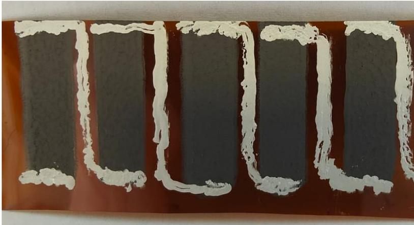
**Fig. 3.12-** Image of single-leg 5% PVDF- $\text{Bi}_2\text{Te}_3$  nanowire FTEG device.
