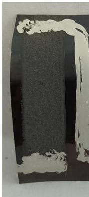
**Fig.5.17-** Image of single-leg PVDF-Bi<sub>0.4</sub>Sb<sub>1.6</sub>Te<sub>3</sub> nanoplatelet + 12 % Te nanorod FTEG device.
