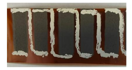
Fig. 3.12- Image of single-leg 5% PVDF-Bi<sub>2</sub>Te<sub>3</sub> nanowire FTEG device.
