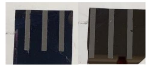
Fig.A.4- Image of 20% PVDF-Bi<sub>2</sub>Te<sub>3</sub> films printed onto (left) SiO<sub>2</sub>/Si and (right) Si wafer pieces.
