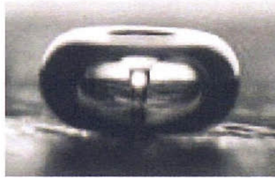
Figure 1.1: Jet formation during the collapse of an oscillating bubble at low pressure ( 0.04 - 0.05 \text{ bar} ) in a 60 - \text{Hz} sound field. The bubble size is ca. 0.2 \text{ cm} . Photograph taken by Prof. LA Crum, University of Mississippi [28].
