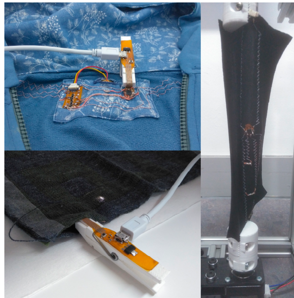
Figure 3. Microcontroller circuit integrated into the collar of a garment ( top left ), a stretchable knitted fabric ( right ), and a custom woven textile ( bottom left ).
