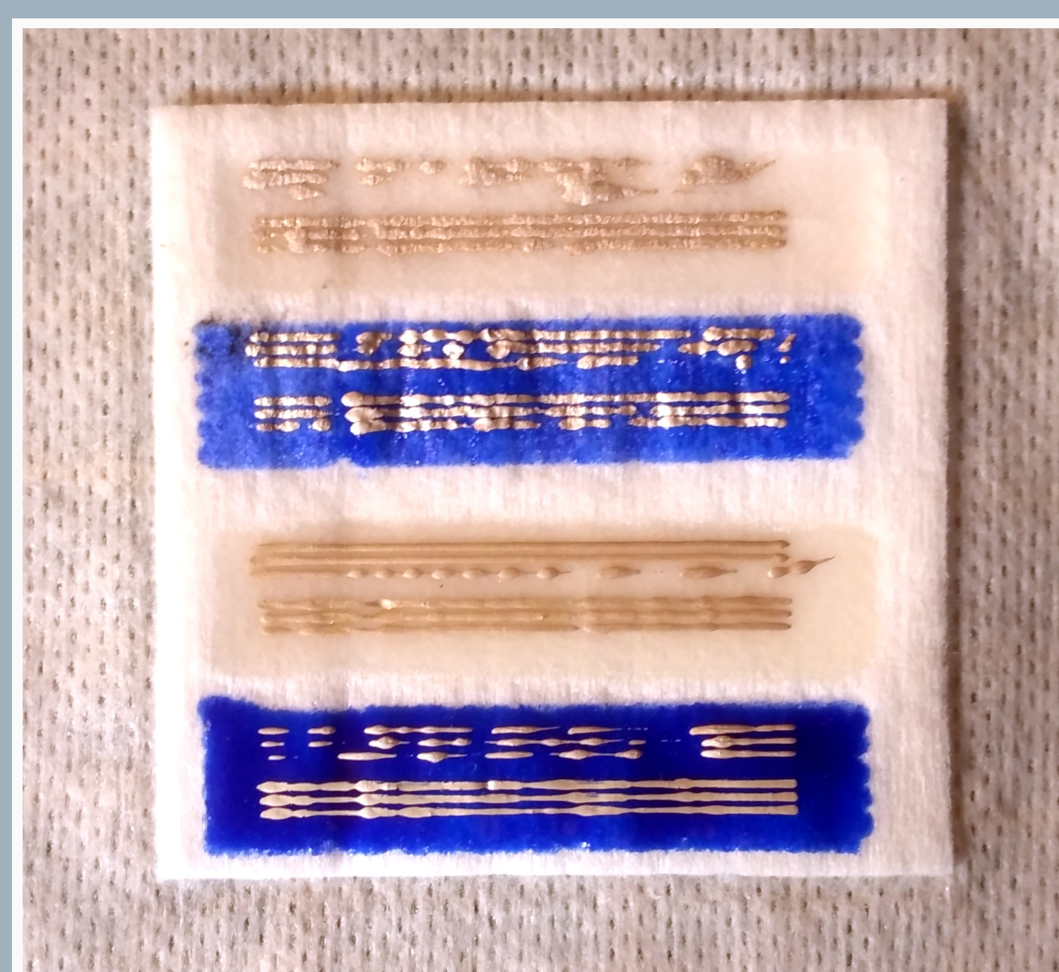
Fig 5. Laser profiling (bottom 3 lines on each strip of interface) provides more reliable printing than printing at a fixed height (top 3 lines).
