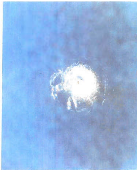
Figure 2.1: Impact damage from a fleck of paint on the Shuttle window. 62
