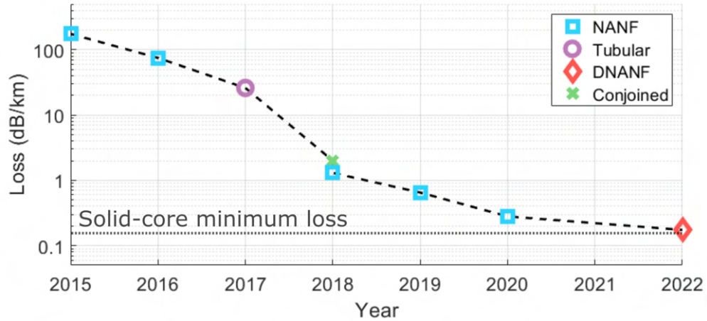
FIGURE 1.1: Reported minimum loss values for fabricated hollow-core anti-resonant fibre between 2015-2022 [21, 22, 31–36] compared to the minimum reported loss in solid-core fibre [23]. Loss is measured at the telecommunications wavelength, 1550 nm, in post-2018 fibres. Minimum loss values for pre-2018 fibre were recorded at shorter and longer wavelengths in the near-infrared and visible.
