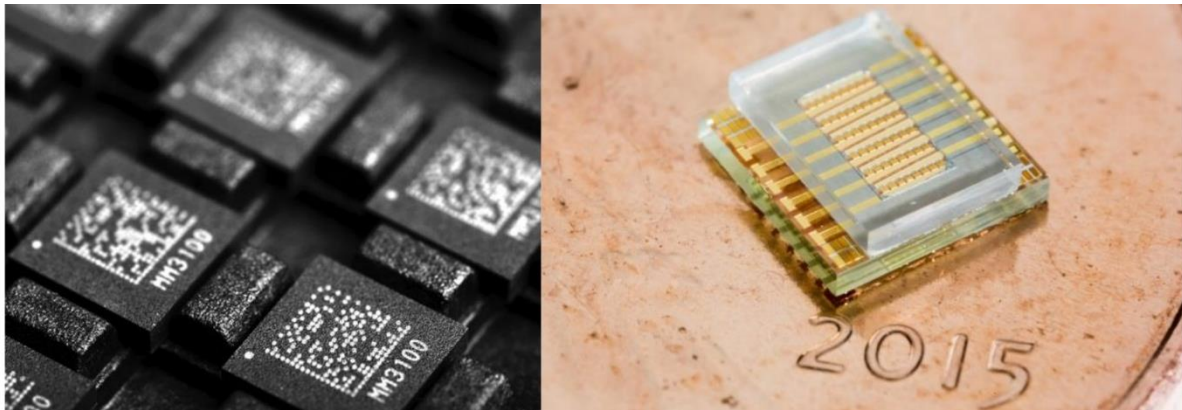
Figure 7-9 - The MenloMicro MM3100 switch packaged (left) and capped wafer showing switch cantilevers (right).
