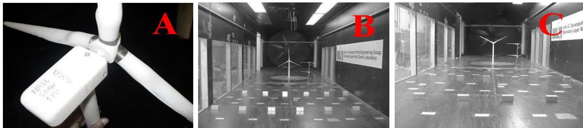
Figure 5: Wind Tunnel test configurations: (A) 1:150 5 MW wind turbine prototype with 1:150 scale, (B) rotor angle = (0°-120°-240°) and (C) rotor angle = (60°-180°-300°), adopted from (Abdelkader 2015).
