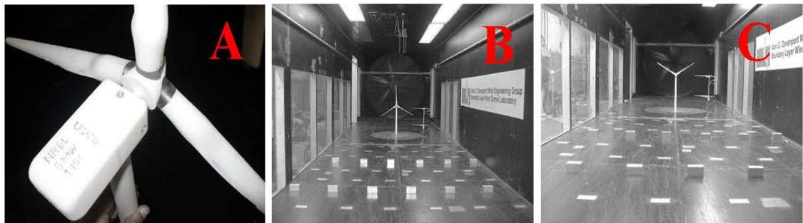
Figure 4-25: Wind Tunnel test configurations: (A) 5 MW wind turbine prototype with 1:150 scale, (B) rotor angle = (0°-120°-240°) and (C) rotor angle = (60°-180°-300°), adopted from (Abdelkader, 2015).
