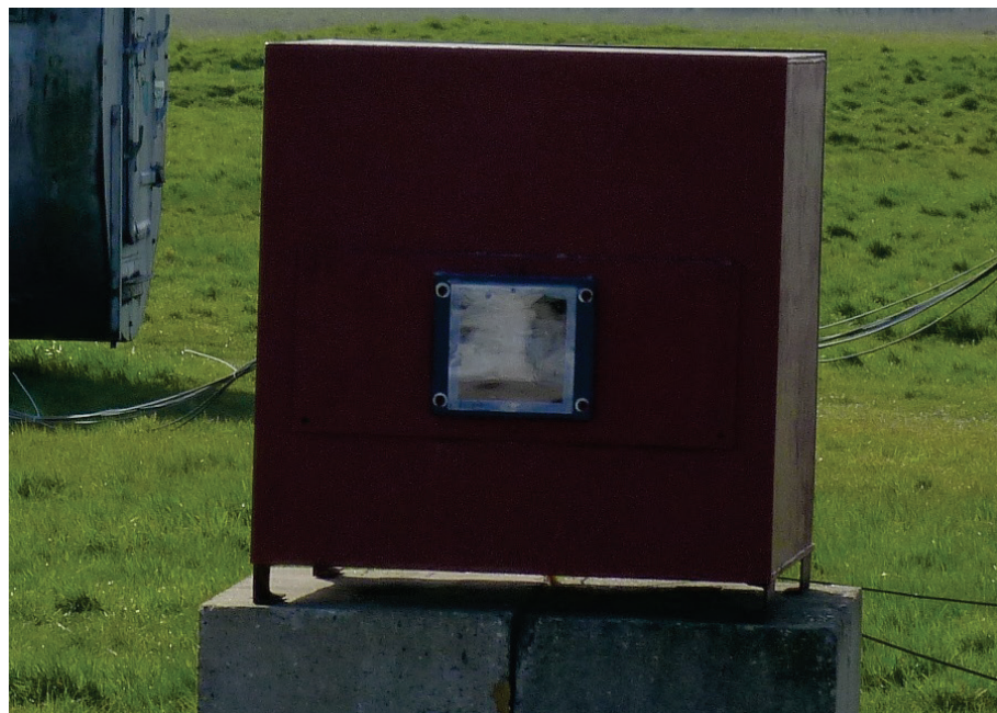
Figure 5.21: Image of armoured housing for high-speed camera.
