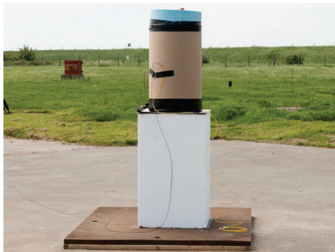
Figure 6.3: Cylindrical charge shape utilised within short-duration blast trial.
