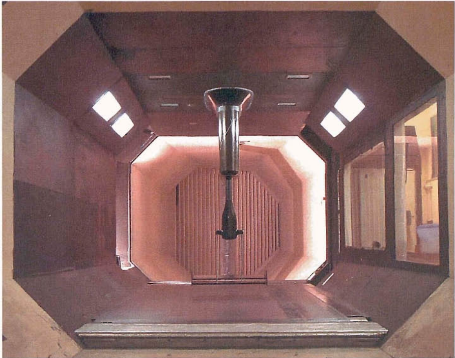
Figure 3.3: Installation of the complete test rig and automated motion system within the 2.1m×1.7m wind tunnel test section.
