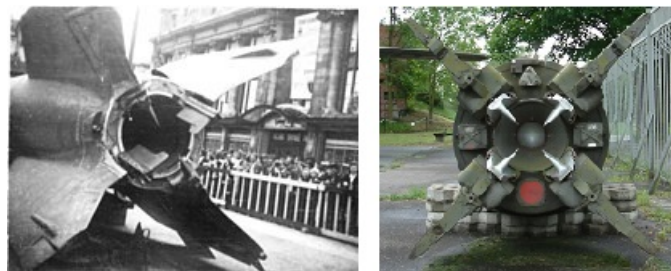
FIGURE 2.3: Jet vane mechanism used in German V-2 and Scud missiles, ( Wikipedia, 2021b,a )
