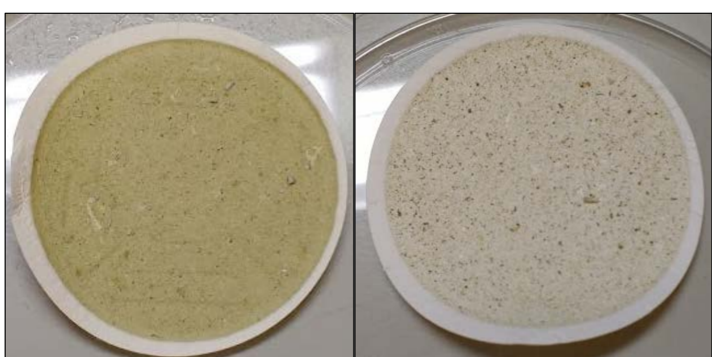
Fig.3: Tissue digestates (n = 3) filtered over 1.2 µm. Left: M. gigas , right: R. philippinarum
