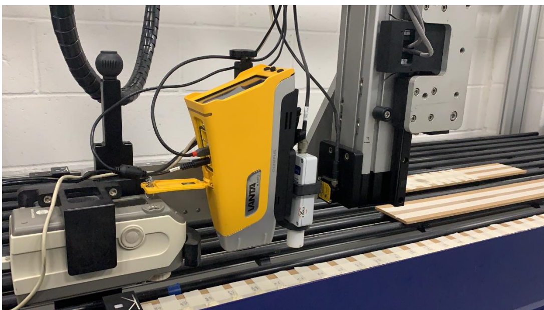
Figure 5.3 Olympus Vanta mounted on a core scanner to analyse the powdered fish muscle samples, which are presented to the instrument in a grid arrangement.
