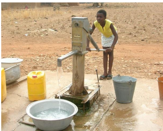
Figure 2-7: Borehole with hand pump (Source: News of the South, 2016)
