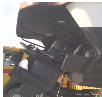
Figure 2. The pair of interceptors and trim tabs were mounted on the high-speed craft, Volcano 71 having sterndrive propulsion system unit.
