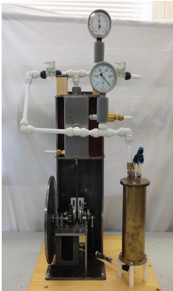
Figure 4-2 Photographed Mk.III condensing engine in the hydraulics laboratory. LEFT: Ancillaries removed. RIGHT: Engine set up for testing.
