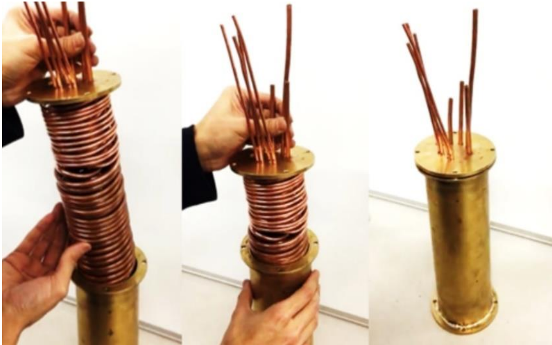
Figure 2-22 Assembly of MK.II coiled shell and tube condenser. Credit: (Ho Chan, et al., 2017).
