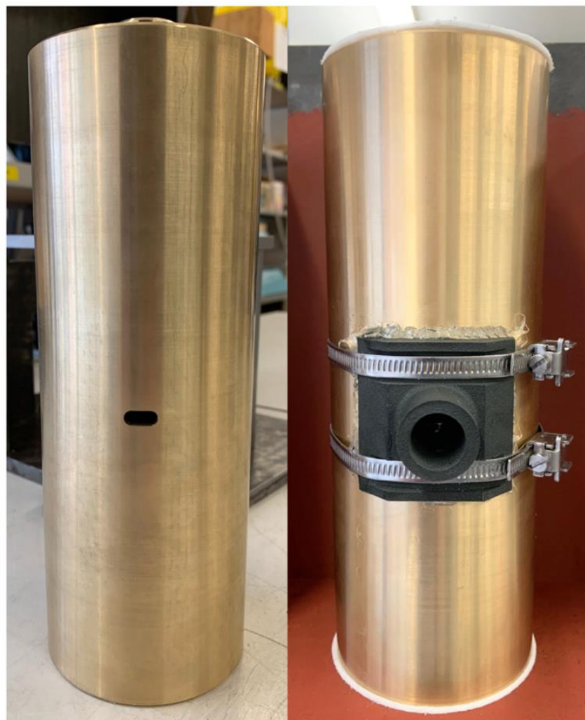
Figure 4-14 LEFT: Mk.III engine cylinder with slot shown. RIGHT: Mk.III engine cylinder with 3D printed exhaust manifold.
