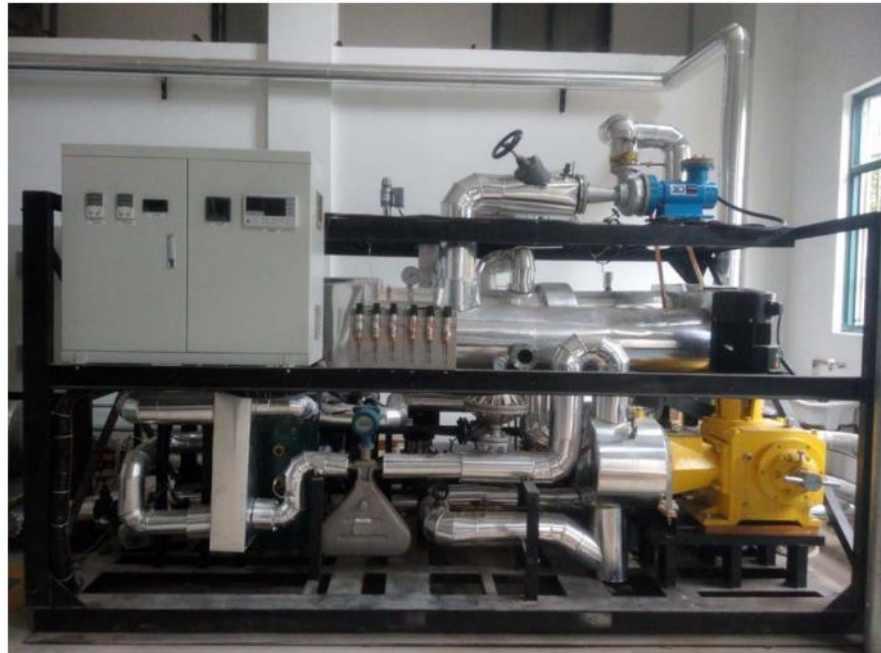
Figure 2-8 Example of a 16.3kW low temperature heat recovery ORC system tested in literature. Note, cooling water circuit not shown in image as it was located on the roof. Reproduced from (Li, et al., 2021) under CC BY.
