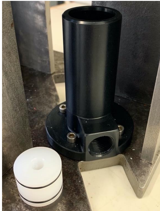
Figure 4-19 Vacuum pump cylinder and piston during assembly.
