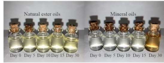
Fig. 2. Discolouration of natural ester and mineral oils during thermal ageing.
