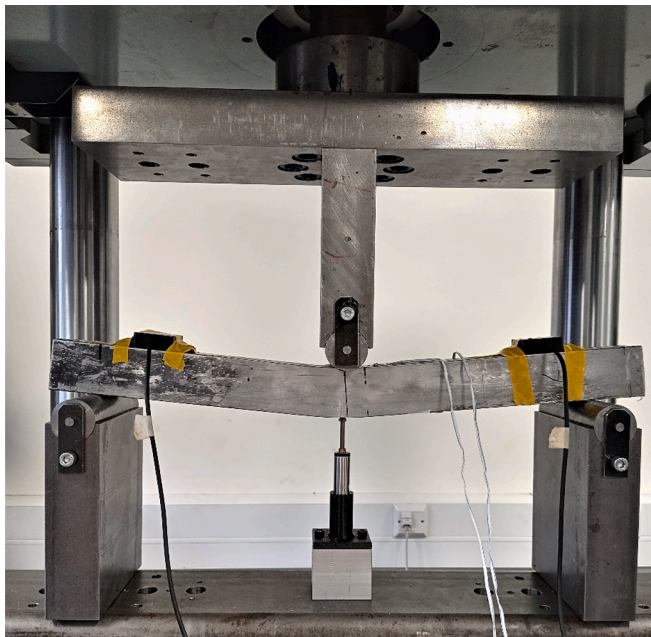
Fig. 8. Typical three-point bending test set-up.
