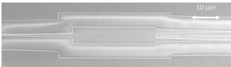
Figure 7-30 SEM image (top view) of fabricated 1x2 MMI of length 32.04 \mu\text{m} .
