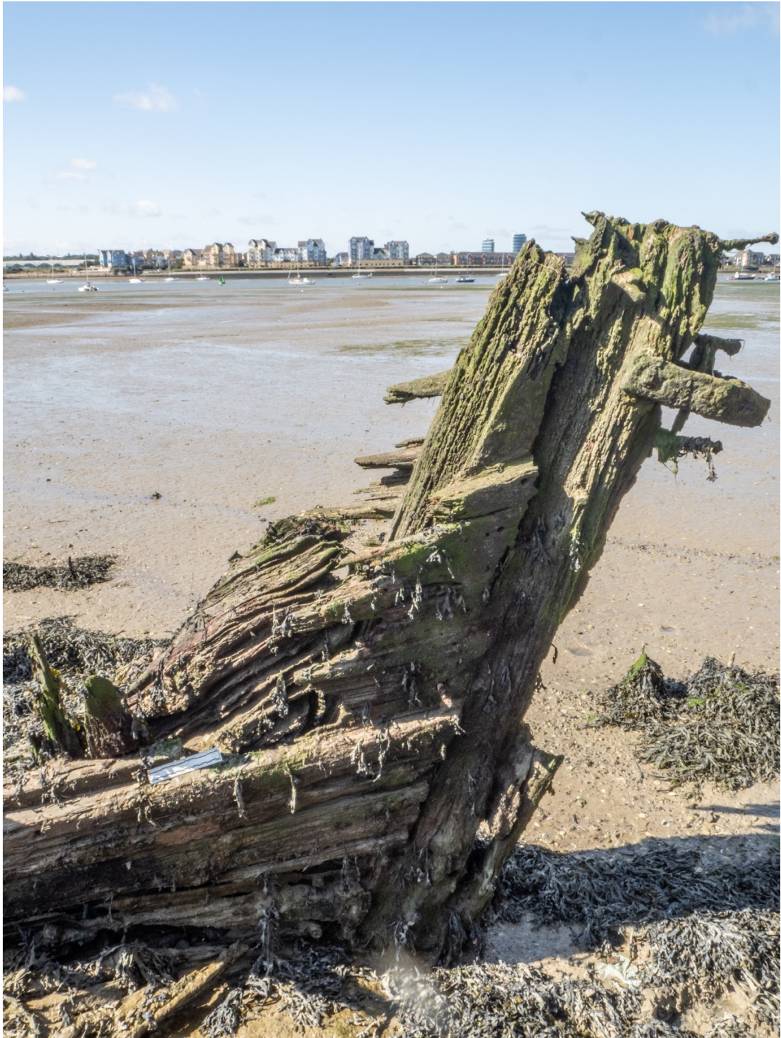
Figure 7.11: The upright sternpost of the ship. There is one rudder gudgeon toward the top of the post and part of the rudder sticking out of the mud at the bottom (Image by the Author).
