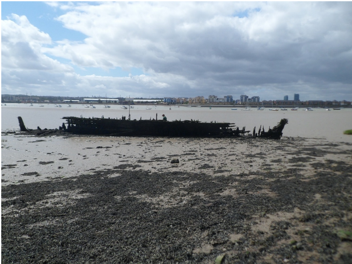
Figure 7.10: Broadside of Rhoda Mary showing the hogged keel as the bow and stern are lower than the middle of the site (Image by the Author).
