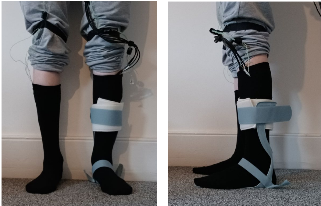
Figure 3.3: Example of a participant fitted with the ES AFO and temperature and humidity sensors, including the thigh bands ensuring the wires were not a tripping hazard.
