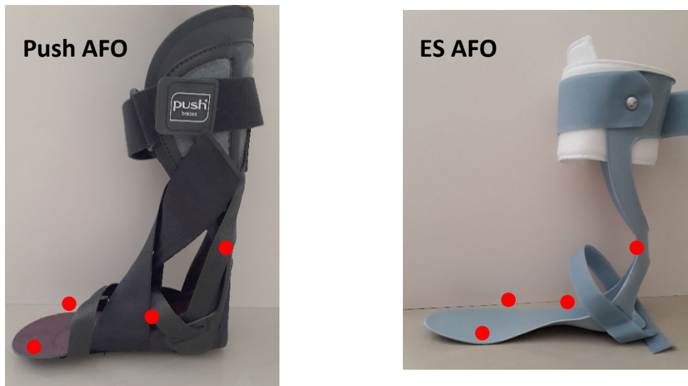
Figure 3.20: Coverage of AFOs compared to combined temperature/humidity sensor locations (indicated with red circles)
