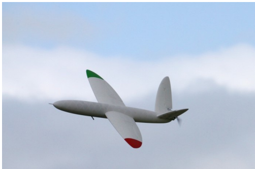
(E) Small UAV: Southampton University Laser Sintered Aircraft (SULSA) (follow link to image source).
