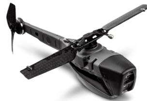
(F) Micro UAV: FLIR Black Hornet PRS (follow link to image source).
