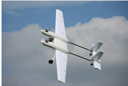
(D) Light UAV: University of Southampton Spotter Light UAS (follow link to image source).
