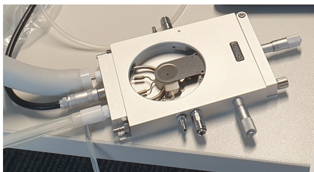
Figure 5-1 An open Linkam THMS600 cooling stage showing the cooling block used for the experiments. The stage is closed and purged with liquid nitrogen via the liquid nitrogen tubes on the left-hand side. A temperature controller is connected to the stage and a PC interface software, which is used to set the temperature profile.
