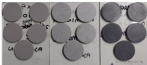
Fig. 1 Coupons (40 mm dia.) attached to a glass plate before being immersed in a natural seawater tank at the Dove Laboratory (Cullercoats Bay, UK). From left to right there are FRC coupons, ACP and uncoated, sanded PVC coupons (control).
