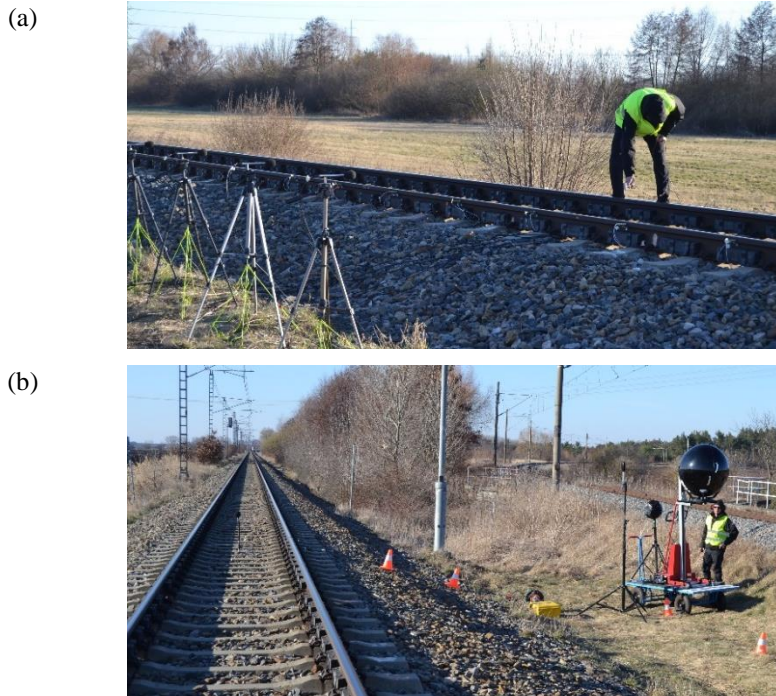
Fig. 1. Experimental set-up. (a) Impact measurements on the track; (b) sound sources used for reciprocal measurements.
