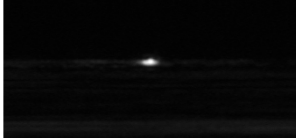
FIGURE 6.14: Mode intensity profile from sputtered thin film bismuth-based rib waveguides.
