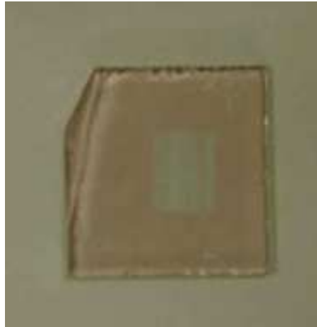
FIGURE 7.4: Photograph of pink sample after poling at 280°C and 1 kV. The bleached (i.e. colourless) region under the anode is well defined by the electrode size.
