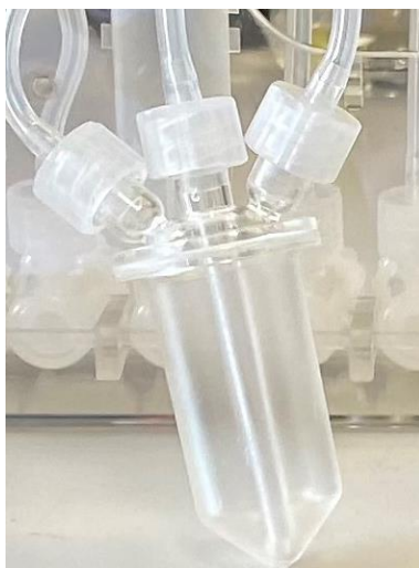
Figure 5.8: A photo of a reaction vessel used on the GE FASTlab, attached to a cassette
