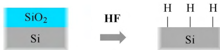
Figure 3.8: The thin native silicon dioxide layer was removed using hydrofluoric acid resulting in a hydride-silicon surface.
