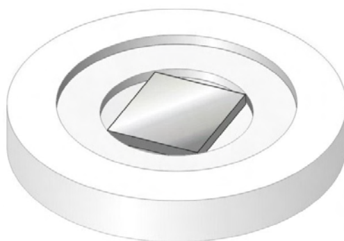
Figure 5.24: The final sample-holder used for experiments was machined from PTFE, with a recess to accommodate the sample and a buffer reservoir. The holder was then sealed using Parafilm tape with a coverslip window in the centre.
