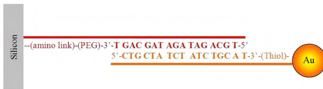
Figure 3.16: Gold nanoparticles featured oligonucleotide sequences complementary to those immobilised on the silicon.
