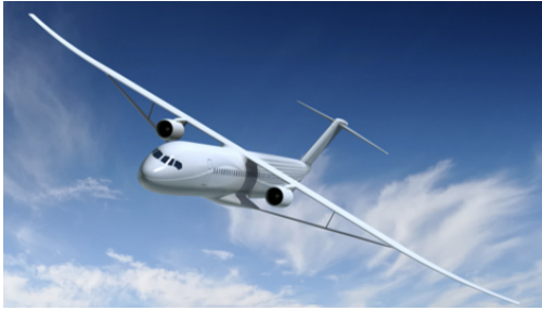
(a) Strut-braced high-aspect-ratio wings, from [49]
