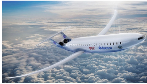
(b) Double-bubble fuselage, high-aspect-ratio wing configuration, from [54, 55]
