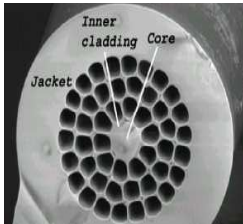
Figure 2.4: Jacketed Air-Clad fibre whose outer cladding is formed by air-holes (here, the inner-cladding diameter is \sim 30\mu\text{m} ) [7].
