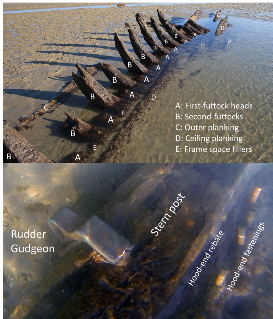
Fig. 4 Detail view of some structural features of Ocean showing the framing timbers toward the bow of the wreck and elements of the stern construction (Arch-Manche: Archaeology, Art and Coastal Heritage 2014).
