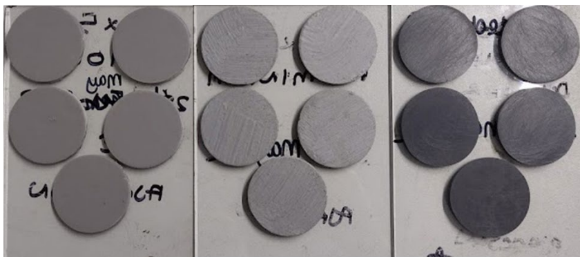
Figure 6-1. Coupons (40 mm dia.) were attached to a glass plate before being immersed in a natural seawater tank at the Dove Laboratory (Cullercoats Bay, UK). From left to right there are FRC coupons, ACP, and uncoated, sanded PVC coupons (control).
