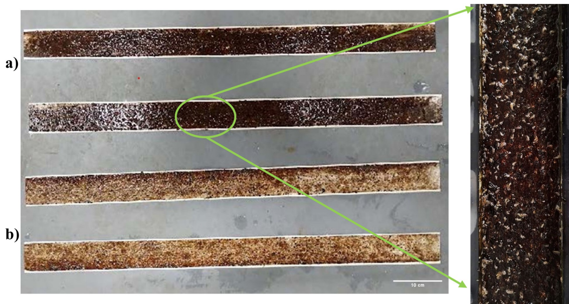
Figure 8-3. Photographs of fouled panels (each measuring 85 cm × 5.5 cm) removed from Hartlepool Marina (UK) where biofilms were grown under a) high flow and b) low flow. The zoomed in area shows evidence of animal fouling, specifically amphipods (white specs), on a HF biofilm.
