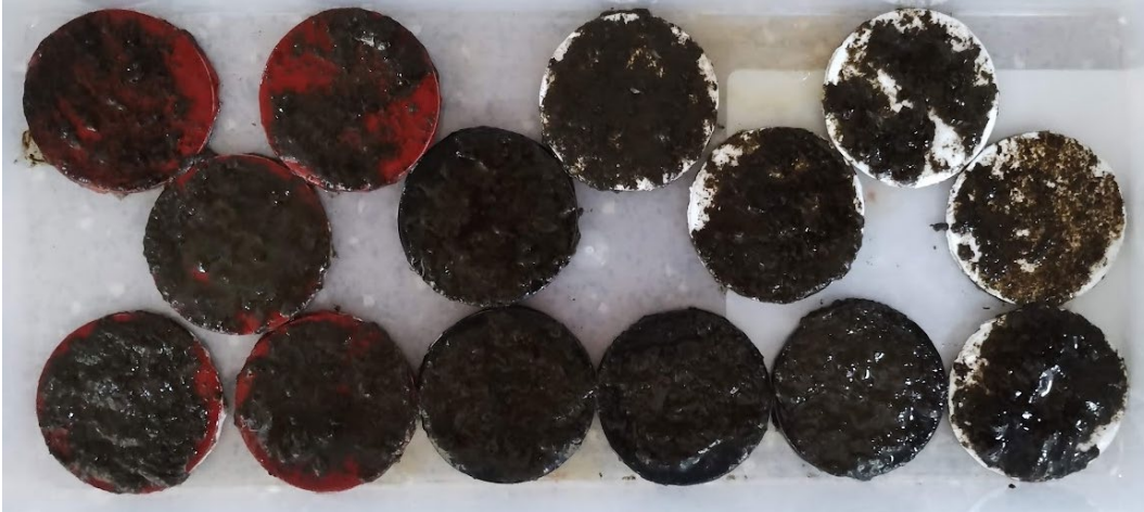
Figure 7-5. Sample of biofilms grown on red, white, and black coupons in Hartlepool Marina (UK).
