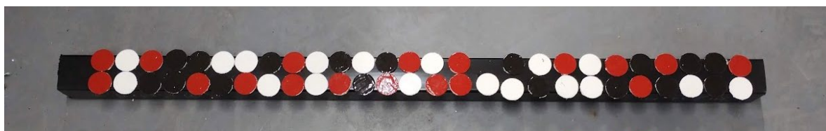
Figure 7-1. 40 mm PVC coupons attached to a square pipe before being immersed in Hartlepool Marina (Hartlepool, UK).
