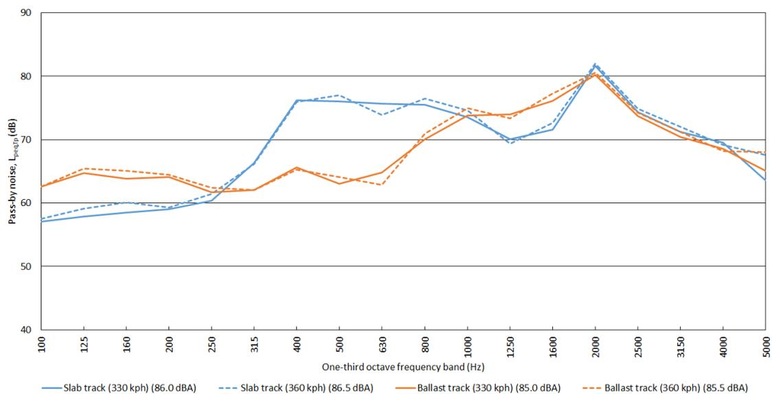
Figure 6: Unweighted sound pressure spectra at 25 m for train running on slab and ballast tracks at 330 and 360 km/h (overall A-weighted values in legend)
