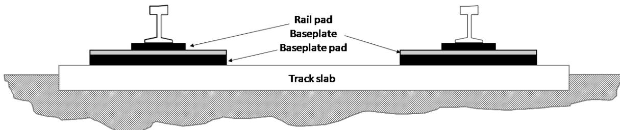
**Figure 1:** schematic of a dual stage rail fastening used on slab track
