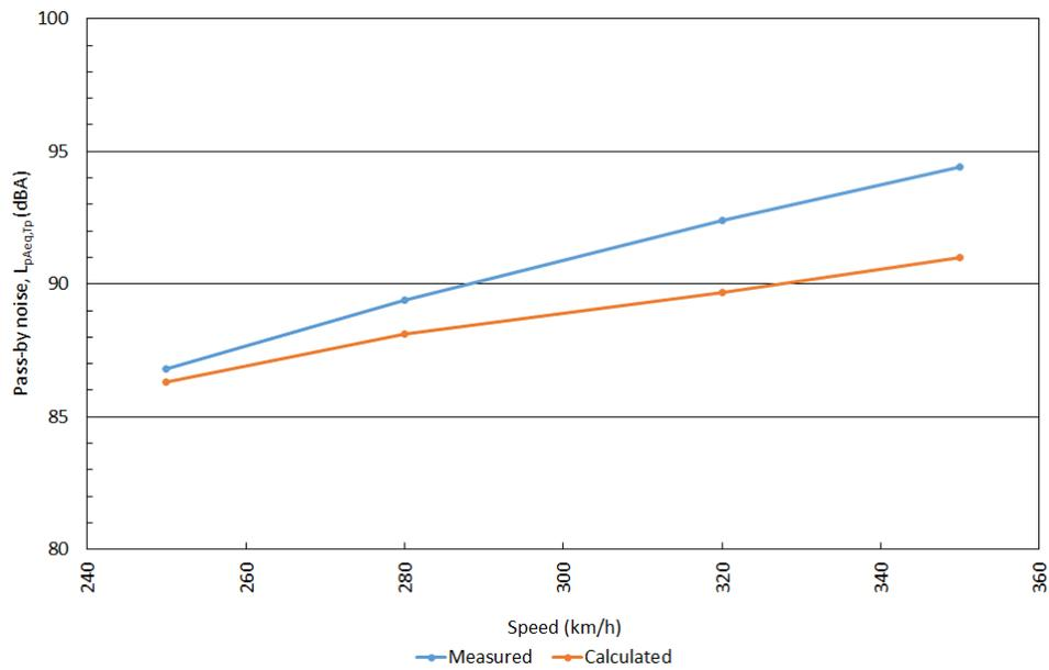
Figure 5: Measured and calculated overall A-weighted sound pressure levels at 25 m with speed, Spanish trial
