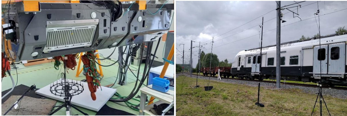
Figure 3: Left: Sound power measurement on a power converter with an acoustic array; right: static measurements of the same equipment mounted on the train.
