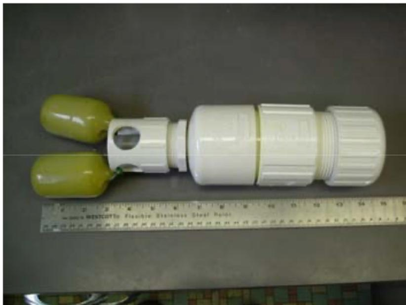
FIGURE 2.9: Design of LRCpH wireless rumen measurement system [29]. A pH electrode from Sensorex was protected from the rumen epithelium by a shroud with holes to encourage rumen liquid contact. The bottom weights helped the capsule sit in the desired position within rumen.
