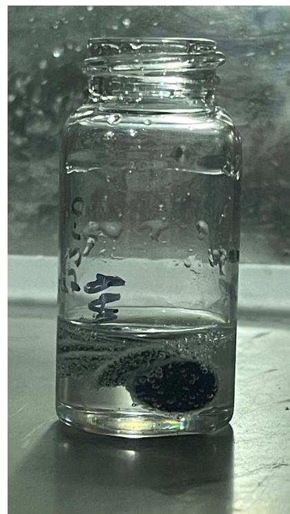
FIGURE 4.4: Textile supercapacitors immersed in polymer electrolyte undergoing vacuum impregnation. Bubbles can clearly be seen on the surface of the electrode and then detach and float to the top of the electrolyte volume.
