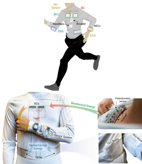
FIGURE 2.9: Schematic and images of the TENG and BFC microgrid. The full system includes energy harvesters/generators, storage and end use applications. The synergistic consideration of the movement and sweat produced via running makes this arguably the most advanced e-textile power module seen in the literature. Image modified from [178]
