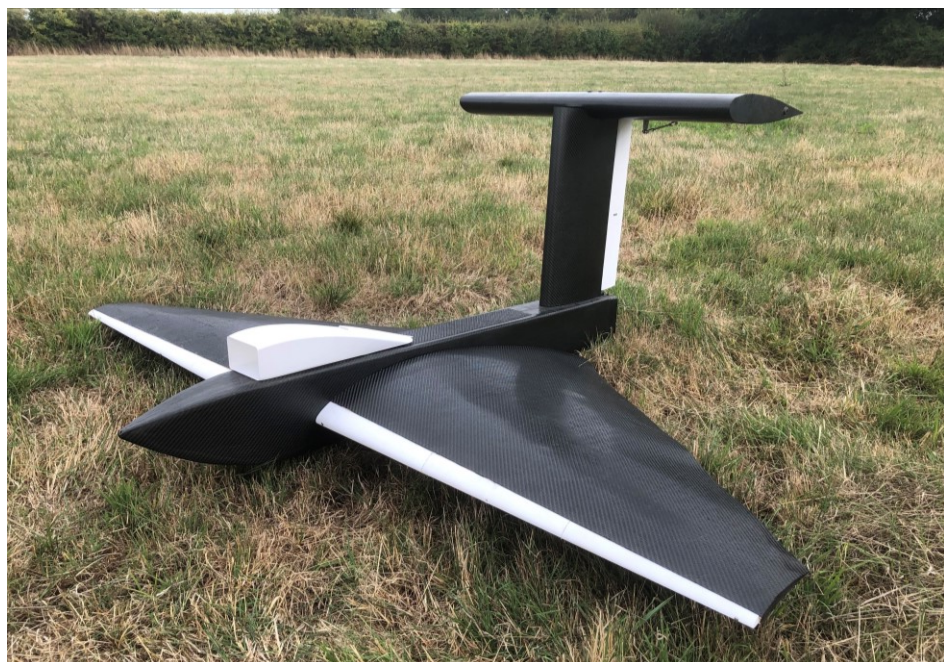
Figure 7.1: Wing in Ground Effect UAV.
