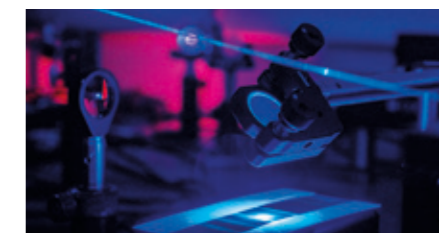
Laser-patterning of a porous paper substrate with a low-power blue laser creating a microfluidic device with a user-defined geometry.
