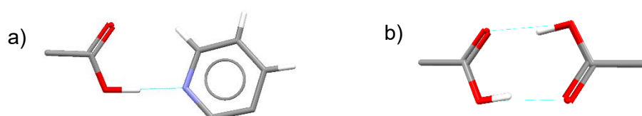
Figure 1.1 Examples of (a) a supramolecular heterosynthon displaying O–H···N hydrogen bonding and (b) a supramolecular homosynthon displaying O–H···O hydrogen bonding
